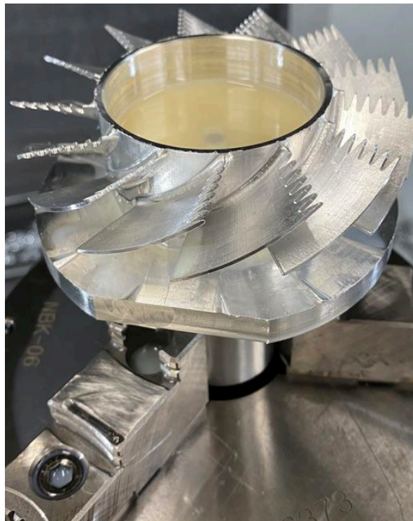
Figure 21 – The manufactured fan with a trailing edge serration, clamped into the 5-axis CNC.
