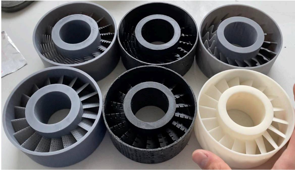
Figure 20 - Top left: Serra-A, top middle: Serra-B, top right: Serra-C, bottom left: Porous-A, bottom middle Slits-A, bottom right – original OGV from Dyson
