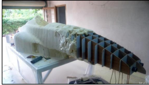
Figure 53: Showing the mould strategy for the bodywork (Ludemann Engineering, 2013).
