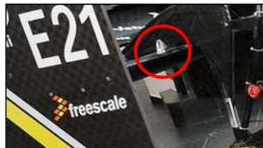
Figure 75: Tu Fast racing swan neck and mounting system highlighted (TuFast Racing, 2017)
